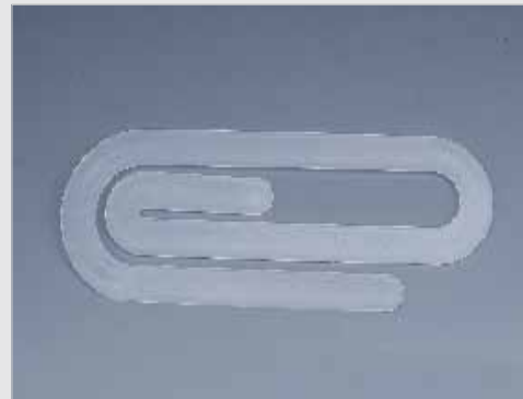
Graphical representation is from the VE900/210 machine, using the standard round ruler test mold. Material POM, cycle time 17.6 s
